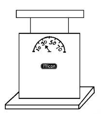
'Micon' Mechanical Cells are simple rugged instruments to read load exerted. Heights are low. It is an economy tool with good accuracy and gives direct reading.
