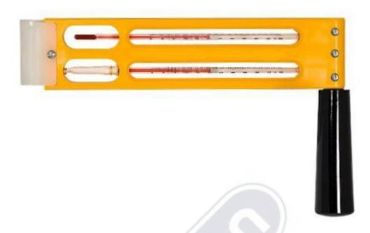
Micon Whirling Hygrometer Consists of two mercury filled prismatic thermometers with least count of 0.5° C and the range 0-50° C and are mounted side by side in a plastic/wooden frame. One revolving handle is fixed to the frame in such a manner that the instrument can be rotated smoothly at about 3 to 4 rev/s to have an air speed of at least 4m/s past the bulbs. One of the thermometers has its bulb covered with a single layer of thin cotton fabric.
